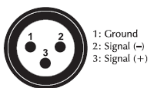
DMX-input XLR mounting-plug:
