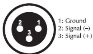
DMX-output XLR mounting-socket:
